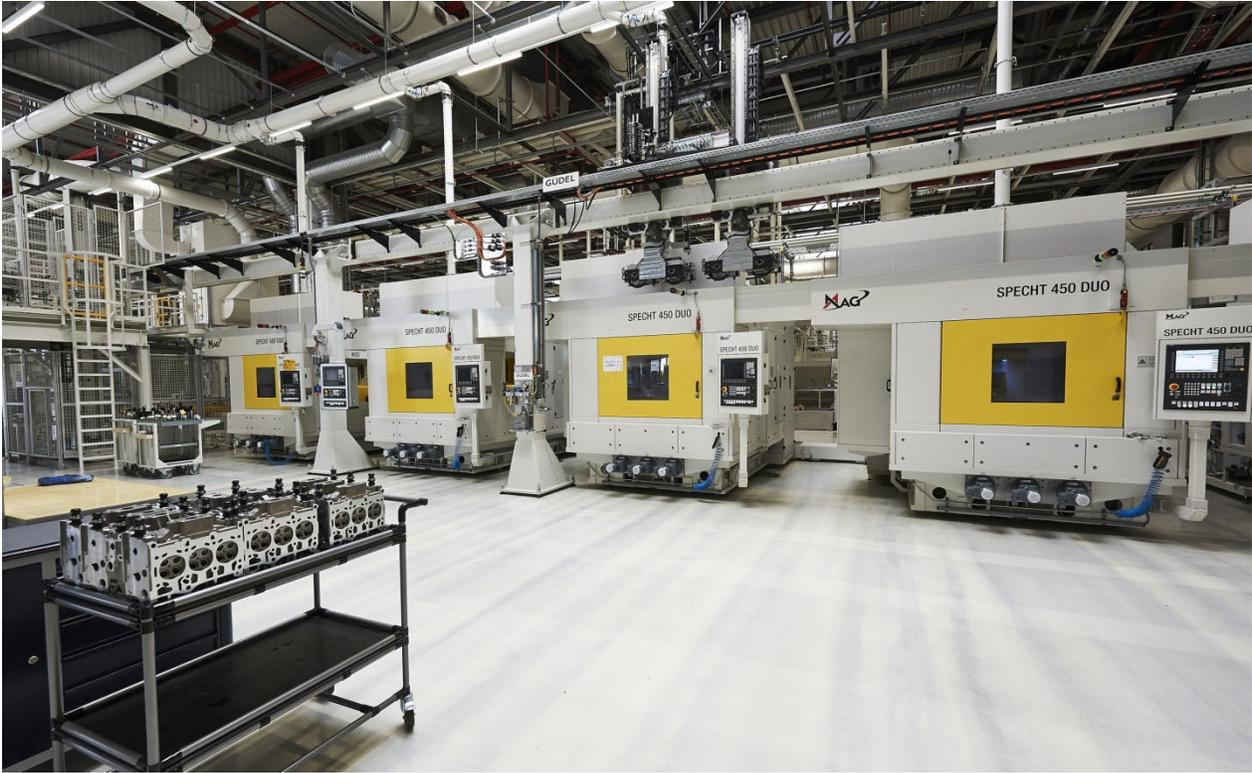
Figure 11: Manufacturing Cell with gantry automation and dual spindle CNC machines DPECHT 450 DUO installed in the customer plant where both components were merged first time physically but commissioned in different locations in a mixed reality procedure
