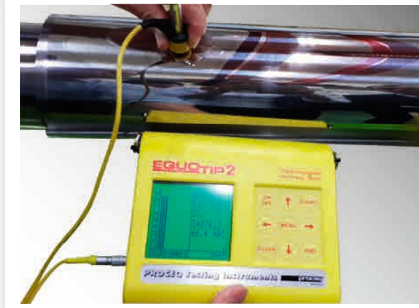
■ The hardness test of W axis
