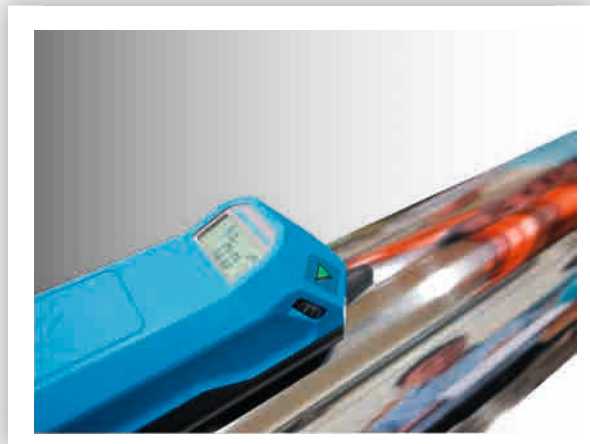
■ W axis surface roughness test
